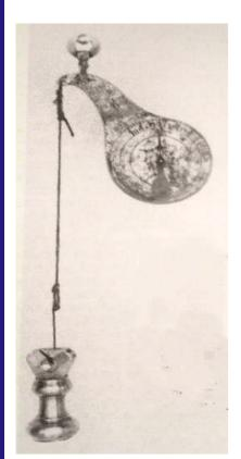
A simple pendulum balance patented in 1863 consisted of a pendulum made from flat sheet brass and suspended from shackle as shown in the figure. The load was applied by a cord and ring. The circular pendulum weight formed a graduated scale at the centre. When a load was suspended from the instrument, the pendulum swung outwards to a position of balance and the pointer indicated the correct weight. These little balances were made for weighing letters and postal packages.
