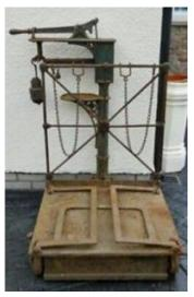
Platform scales were originally fitted with loose - weight steelyards and with these, the major portion of the load is balanced by loose proportional weights and a small sliding poise serves to balance and indicate the odd pounds and ounces.
