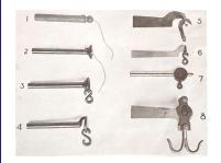
Figure shows stages in the evolution of knife edge, and of the methods of forming or fixing it in the various types of beam ends, such as the swan - neck, the box end, and the dutch end.
