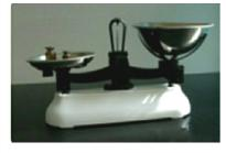
Not until the beginning of the nineteenth century did the scale makers apply this principle to the balance, but since then the Roberval enigma has formed the basis of many counter scales
